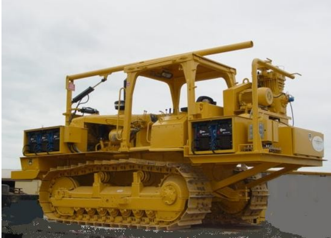
Caterpillar D6E Tractor Shown with (5) Miller XMT 350 welders
