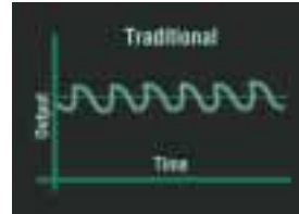
Traditional weld control is more variable around the desired output.
