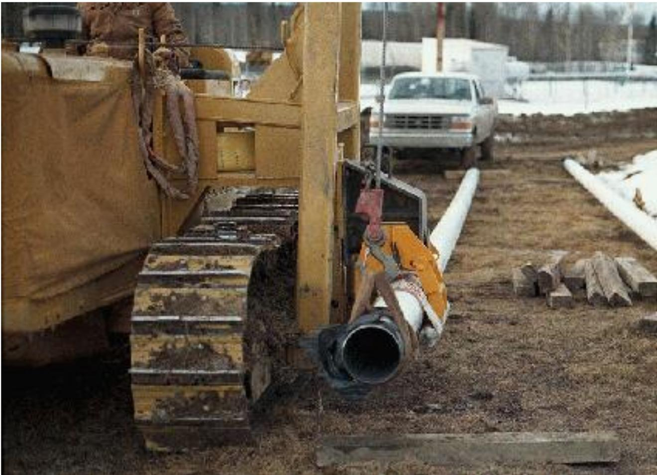
Just take off the segmented tractor bending shoe springs and rail by removing the pin from the tractor bending shoe adapter. Then re-pin the spring shoe to the same location.
