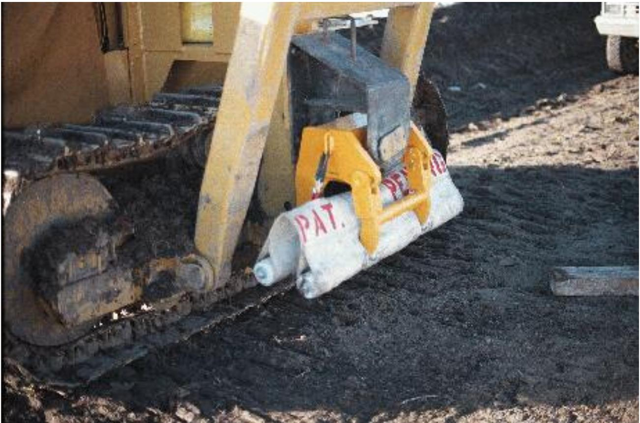
The Spring Shoe Bender can be used to **slip bend** concrete coated pipe with **no damage** to the concrete coating. Since its introduction in 1996, the Spring Shoe Bender has become the **bender of choice** in Western North America, almost completely replacing traditional benders.
