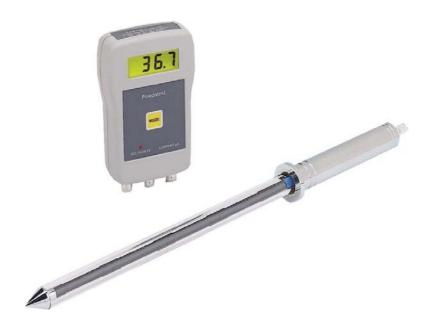
This instrument is designed specifically for testing the output voltages of any make of DC Holiday Testers (DC Spark Testers, Jeep Testers) and High Voltage DC Power Supplies.
