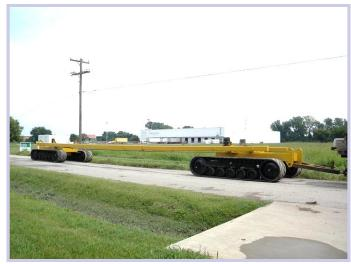
The Challenger Services trailer utilizes the Rubber Track design providing more flotation and stability. The rubber tracks are mounted with a bogie suspension. Brakes and/or hydraulic motors are available as an extra cost option .The trailer has a 90,000 lbs. net pay-load capacity. This configuration can be used for pipe or general cargo.
