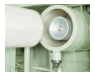
**Two-Stage Air Filter with Safety Element** Provides maximum protection for engine and compressor, thereby lengthening equipment life.
